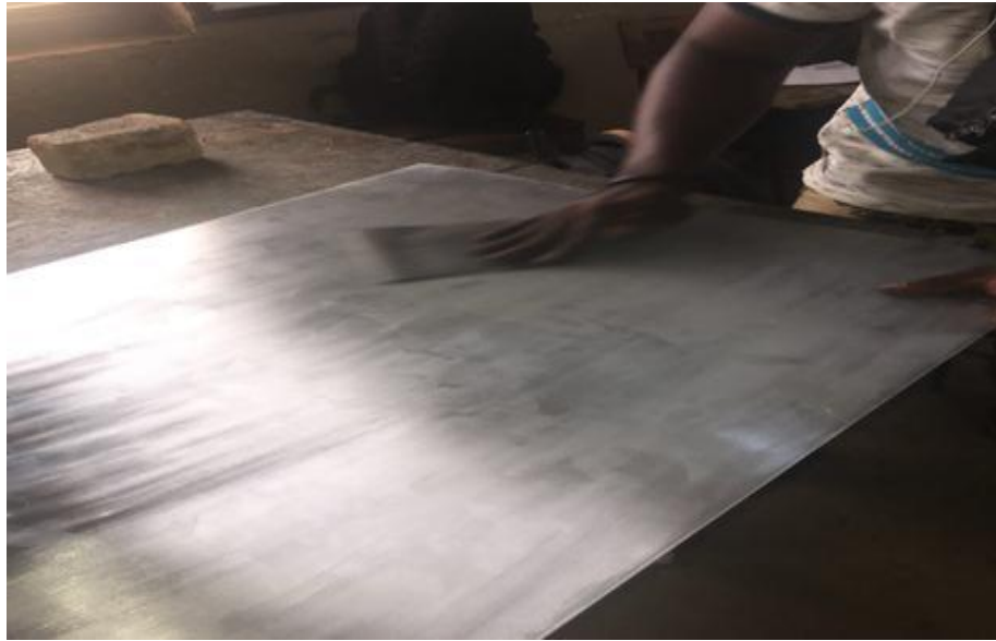
Figure 5: Aluminium sheet scratched to be annealed and worked on for domes
