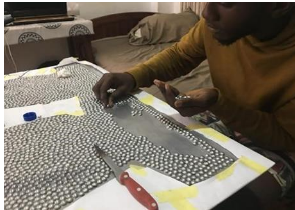
Figure 9: Arrangement and sticking the dooms on the support with epoxy
